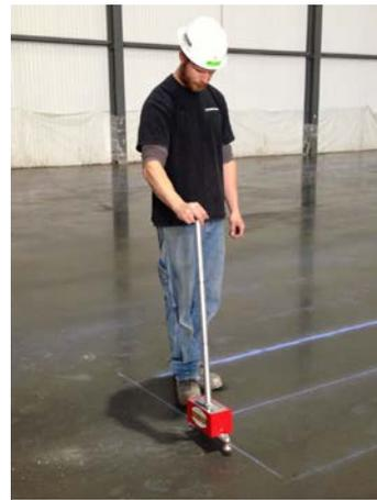
Figure 2: Slab profiling instrument
