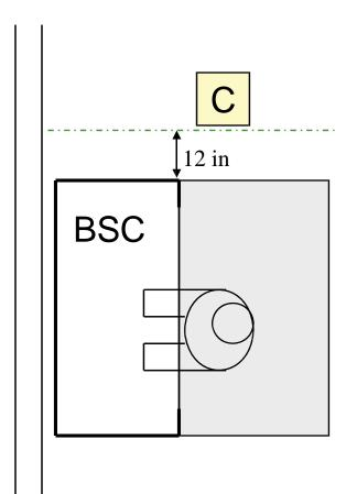
**DO** Maintain a distance of 12" to columns to avoid disturbance to BSC airflow.
